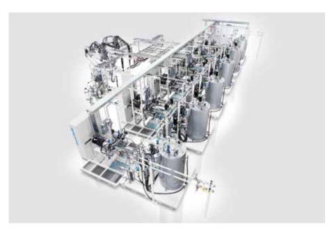
12-component metering machine with two pouring robots
