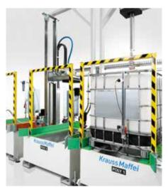
Container station for preconditioning PU components
