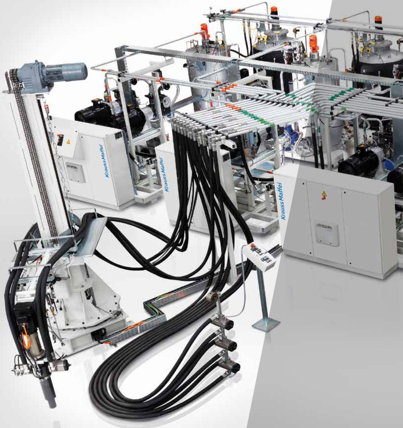
F Series for reaction-casting under low pressure (lower output rates)
