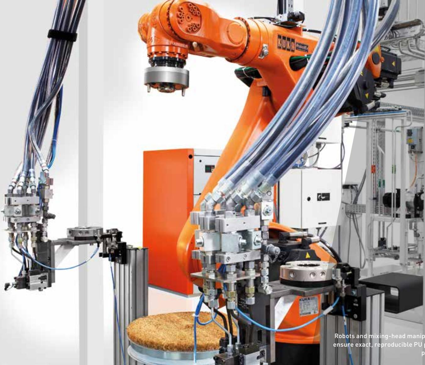
Robots and mixing-head manipulators ensure exact, reproducible PU pouring patterns
