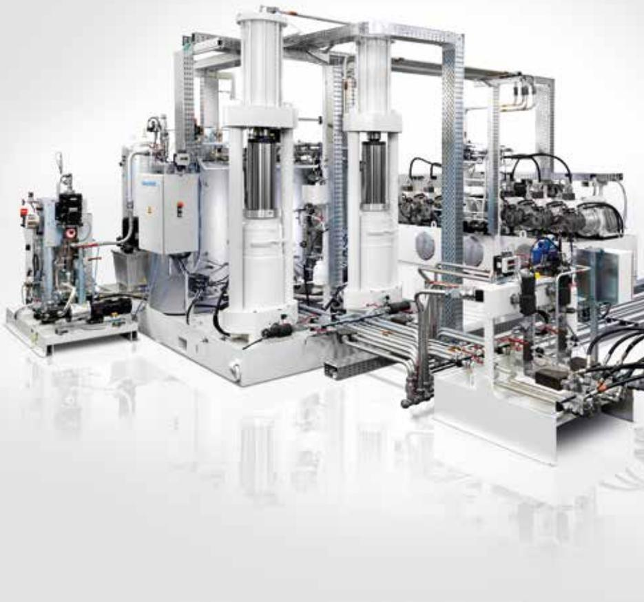
Comet metering machine with hydraulically driven pistons
