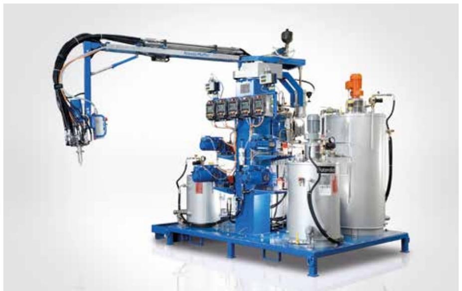
F Series for reaction-casting under low pressure (lower output rates)
